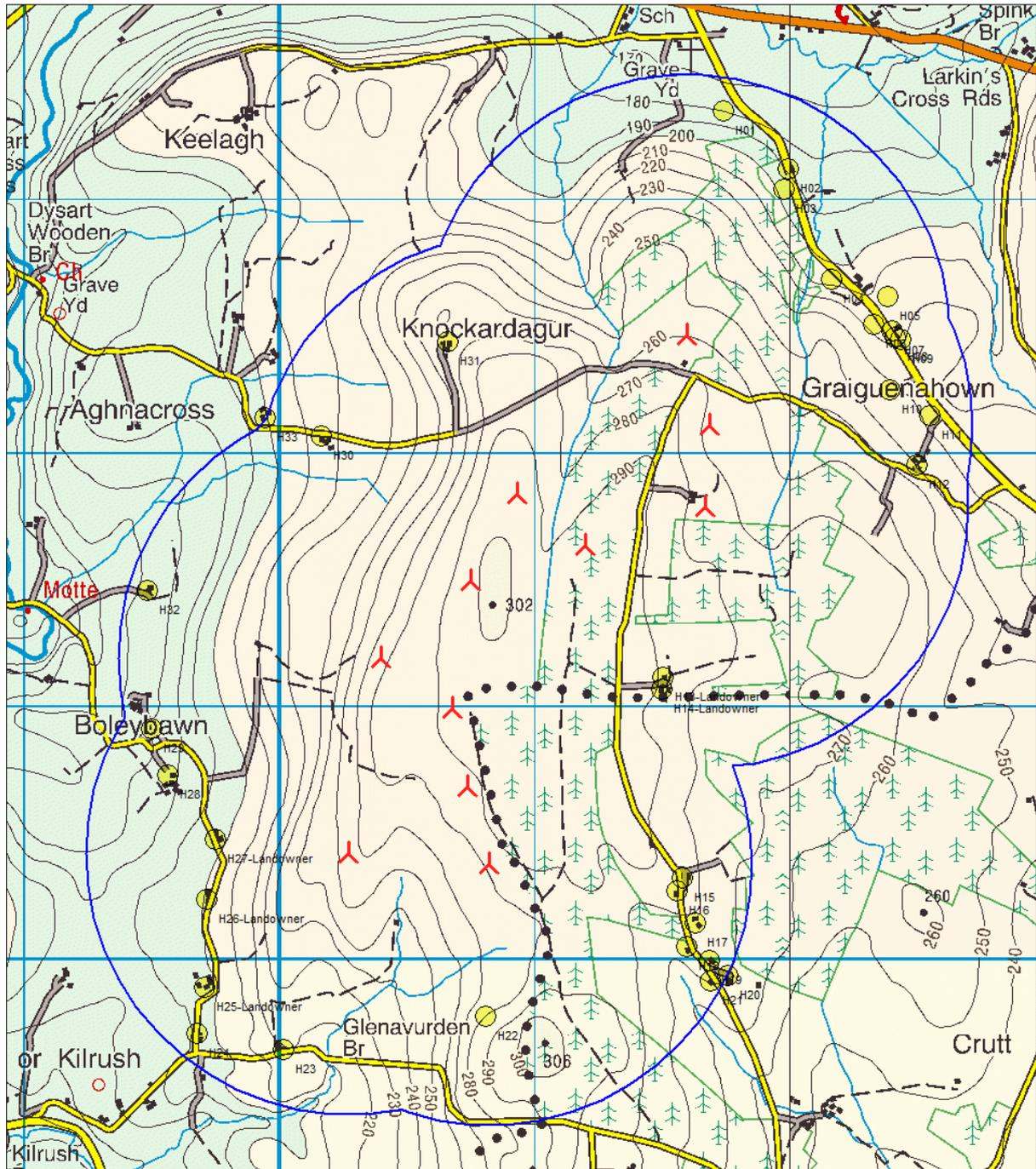
**Figure 11.1: Setback map to dwellings/properties within 1,030m radius (10 rotor diameters) of proposed wind turbines**
