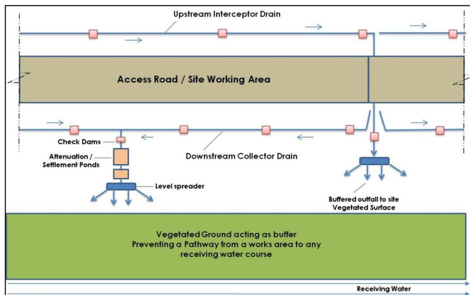
**Plate 6.2: Schematic of Proposed Site Drainage Management**
