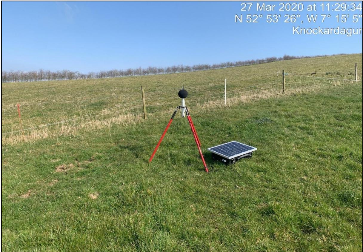
**Figure 11.2: Noise Measurement Equipment**
