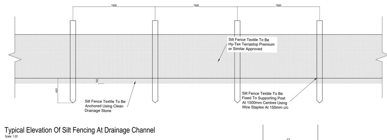
Typical Elevation Of Silt Fencing At Drainage Channel
