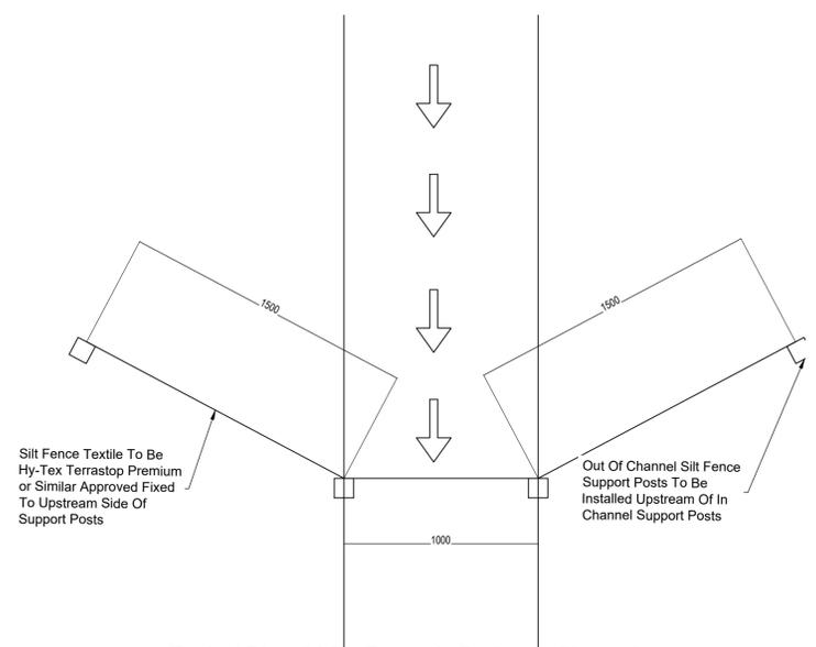
Typical Plan Of Silt Fence At Drainage Channel
