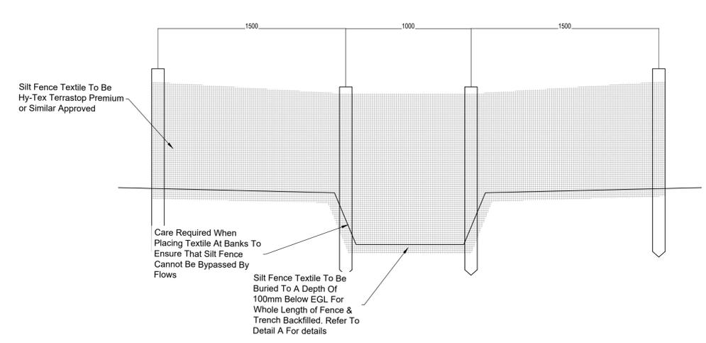
Typical Elevation Of Silt Fencing At Drainage Channel
